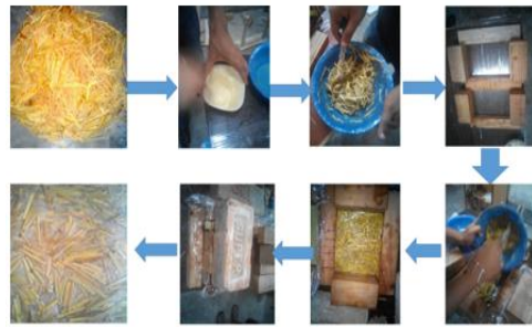
Figure4. complete sequential process for fabrications (a) Fibers (b) Forming the mold (c) Mixing resin and fiber in appropriate proportion (d) Pouring mixer into the mold (e) Pressed to force the air gap to remove any excess air present and kept for 72 hours (f) Fabricated composite
