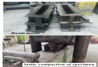
Figure5. Preparations of Beam specimens
