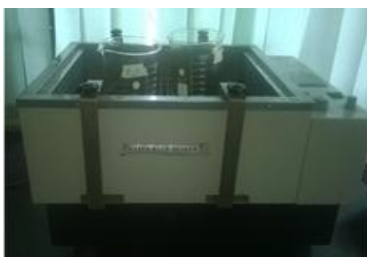
Figure5. Water Hyacinth Extract Subjected to Laboratory Water Bath Shaker
