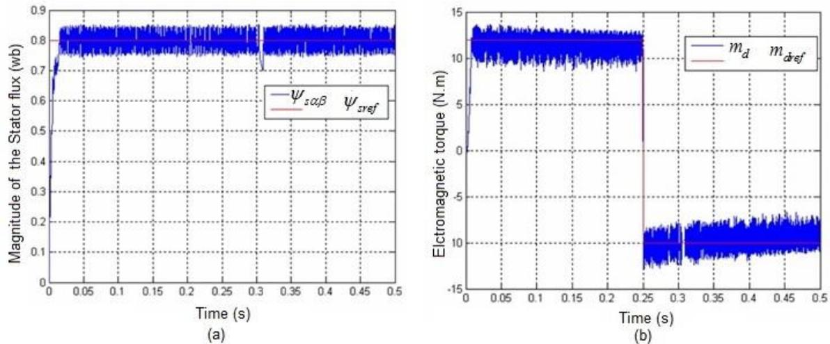
**Figure9.** (a) Simulation results of stator flow estimated, and (b) Electromagnetic torque estimated by the proposed DTC algorithm
