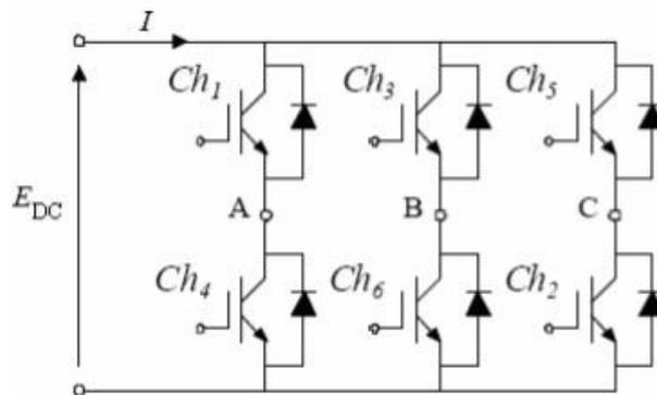
Figure4. Scheme of voltage source inverter
