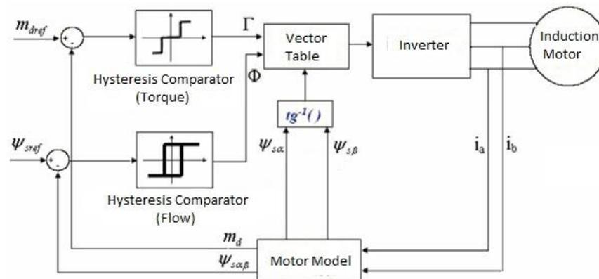
Figure6. Structure of direct torque control system
