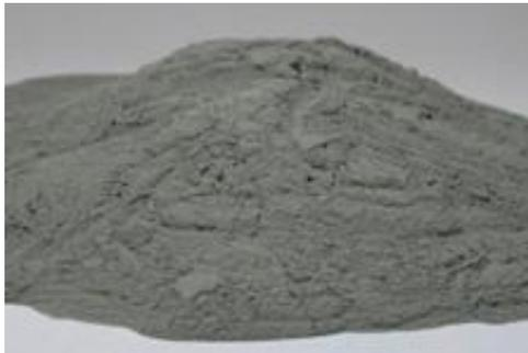
Figure2. Aluminium Powder (20 micron)
