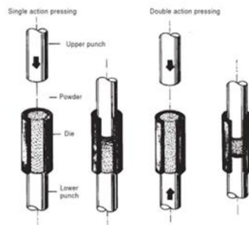
**Figure 1.** Uniaxial Die Compaction of Metal Powder [10]
