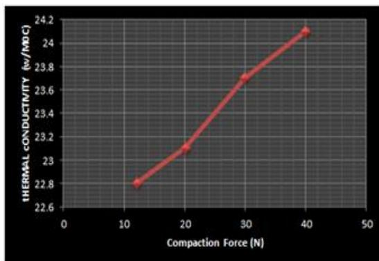
**Figure8.** Plot of Thermal Conductivity against Compaction Force
