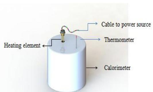
Figure5. Experimental Setup
