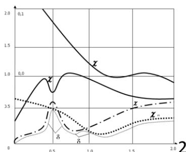
Fig4. Dispersion curves of phase velocities  $\chi_{R1}$ .
