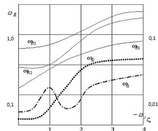
**Fig2.b.** Change in complex eigen frequencies from the wave number. b) dissipative inhomogeneous mechanical system;
