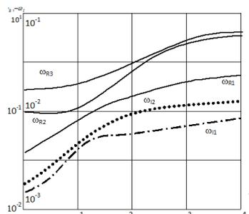
**Fig2.a.** Variation of complex Eigen frequencies from the wave number.
