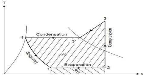
Fig1. T-S diagram of refrigeration cycle
