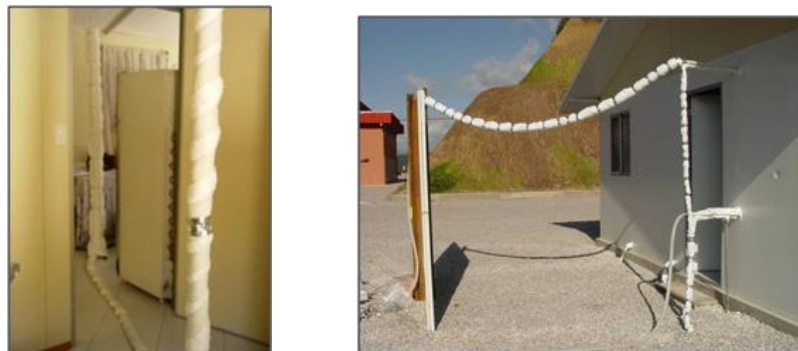
Fig4. Instrumentation - (a) gas collectors located close to the B2 barrier; (b) thermocouple trees inside the prototype.
