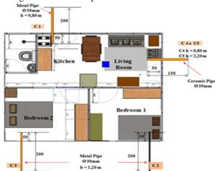
Fig5. Distribution and location of gas collectors.
