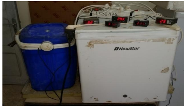
Fig2. Domestic Refrigerator with Water Heater Tank photograph
