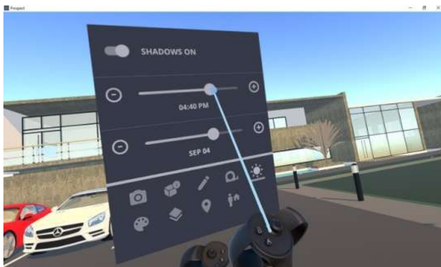
Figure8. Simulation daylight change and shadow movement in Prospect with Oculus Rift
