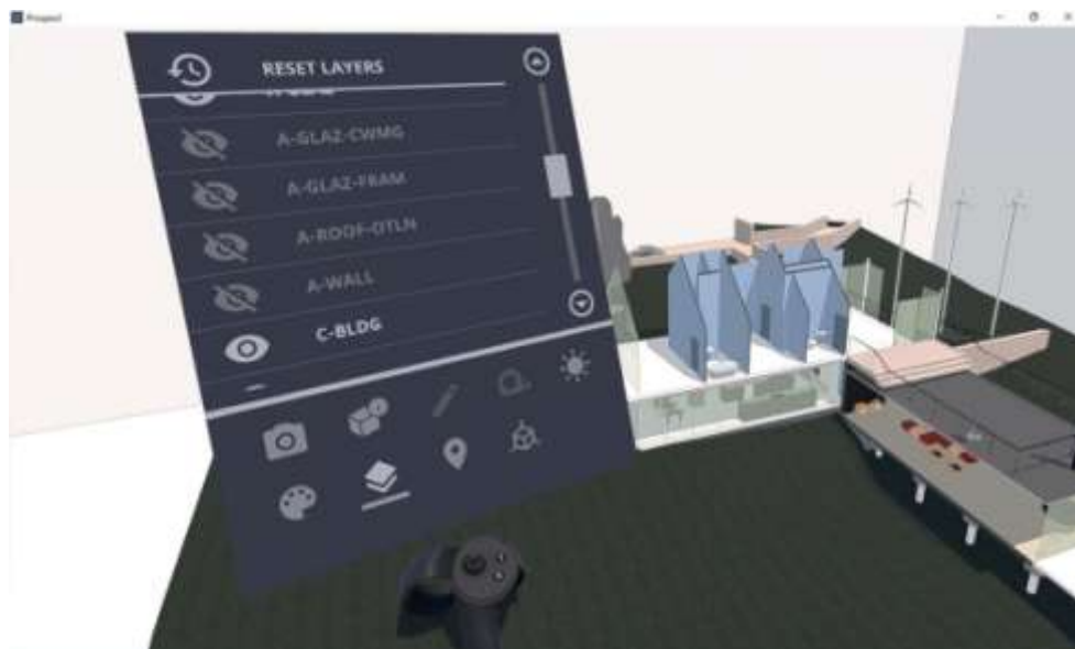
Figure5. A miniature model with various layers turned off in Prospect with Oculus Rift
