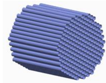
Fig.4.4 Comb structure Capillaries
