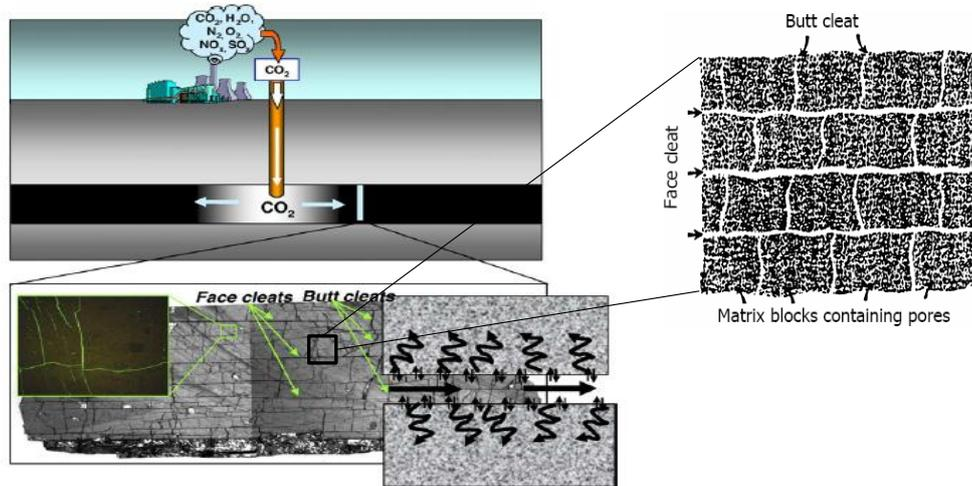
Fig1. Schematic representation of coal seam CO<sub>2</sub> sequestration (modified after Ozdemir 2004)
