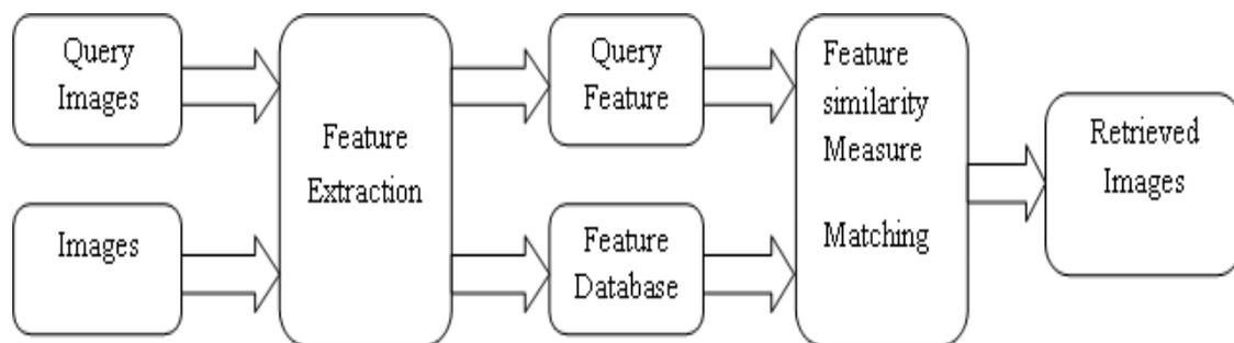
Fig2. Diagram of the Image Retrieval System
