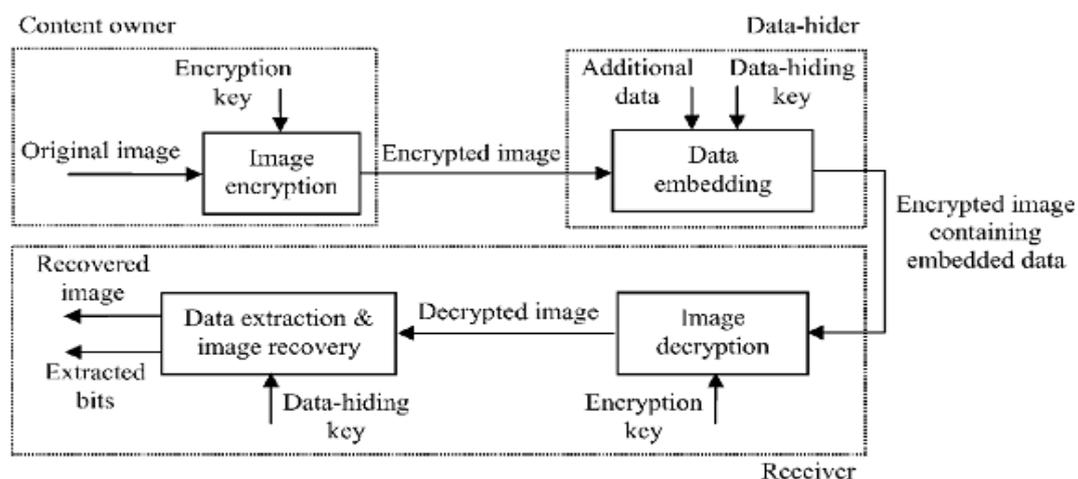
**Fig3.1.** Sketch of non-separable reversible data hiding in encrypted image.
