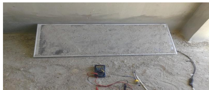
Fig11. Photovoltaic panel with full accumulation of dust and shadow indoor
