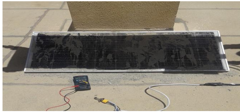
Fig9. Photovoltaic panel with dust and shadow outdoor
