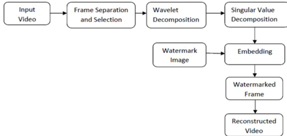
Figure1. Block Diagram for Proposed System
