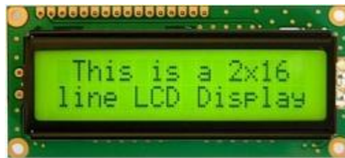
Figure5. 2x16 Line Alphanumeric LCD Display
