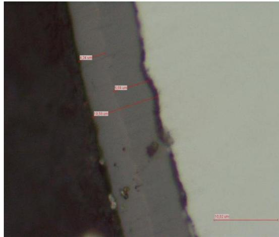
**Fig4.** Scale thickness on sample 1 which laying head temperature is 850°C and cooling rate is 0.50 °C/s seen by light microscope with magnification (1000x)
