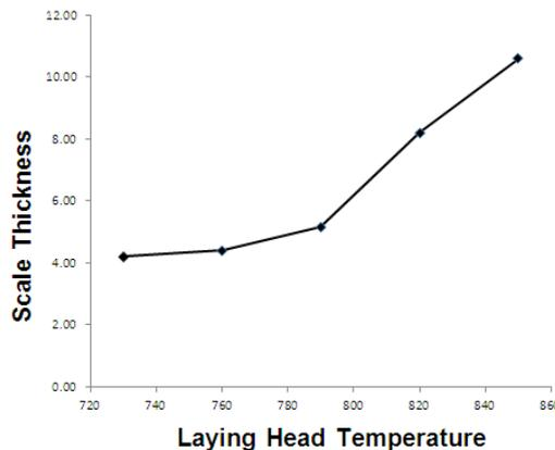
Fig3. Graphics of laying head temperature and scale thickness
