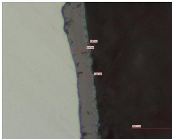
**Fig5.** Scale thickness on sample 5 which laying head temperature is 730°C and cooling rate is 0.50 °C/s seen by light microscope with magnification (1000x)
