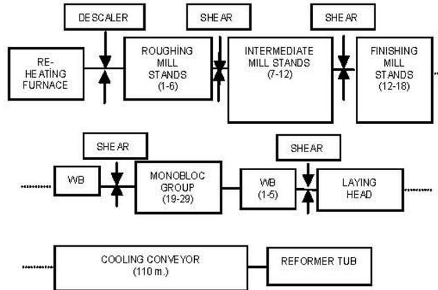
Fig2. Layout of wire and rod mill
