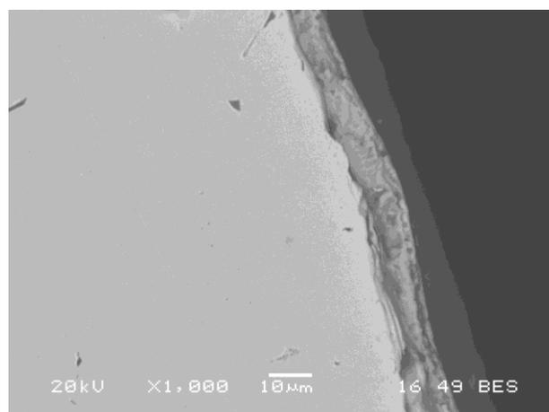
**Fig6.** Scale thickness on sample 5 which laying head temperature is 730°C and cooling rate is 0.50 °C/s seen by SEM-BES with magnification (1000x)
