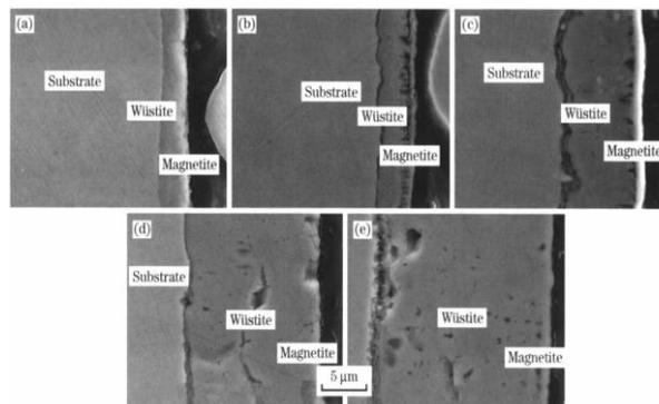
**Fig1.** Oxide scales formed at different temperatures for 15 s. a) 800 °C b) 850 °C c) 900 °C d) 950 °C e) 1000 °C [5].
