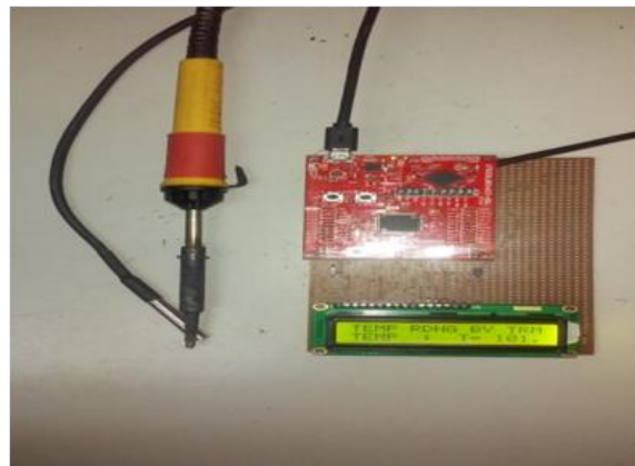
Fig6. Thermocouple interfacing with MSP430F5529 when Power is on and displays the room temperature
