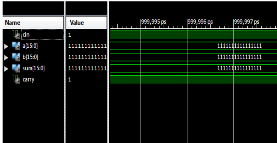
Fig10 (b). 16-bit Regular Sqrt CSLA
