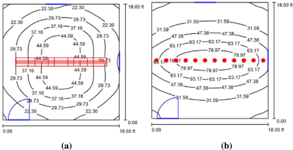
Line Arrangement of Fluorescent Lamps (A) And Led Lamps (B)
