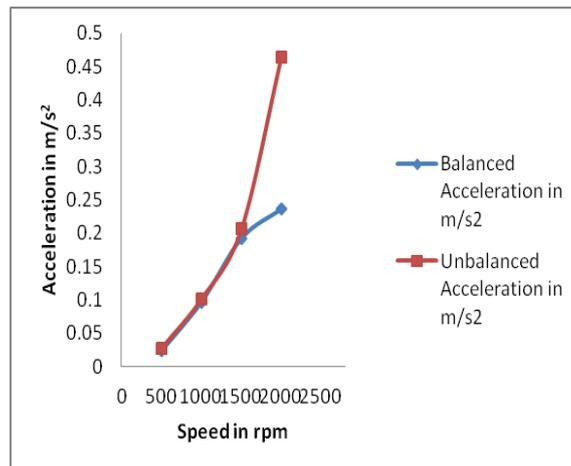
Figure5. Graph for comparison of balanced & unbalanced horizontal position
