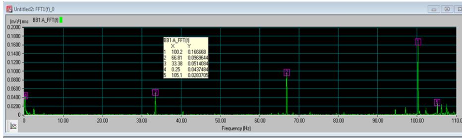
Spectrum at Plummer block no.1 unbalanced 2000 rpm Axial
