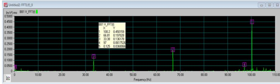
Spectrum at Plummer block no.1 unbalanced 2000 rpm Vertical
