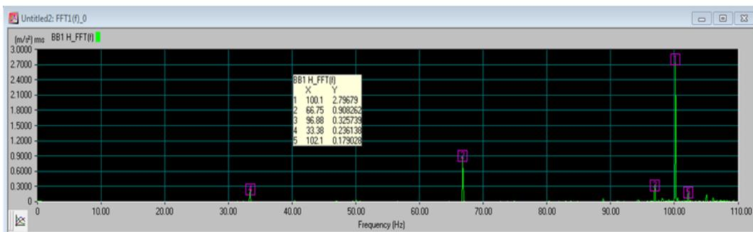
*Spectrum at Plummer block no.1 balanced 2000 rpm Horizontal*
