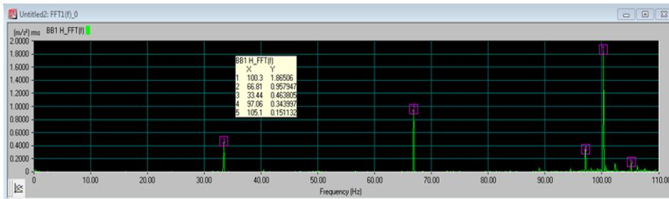
Spectrum at Plummer block no.1 unbalanced 2000 rpm Horizontal
