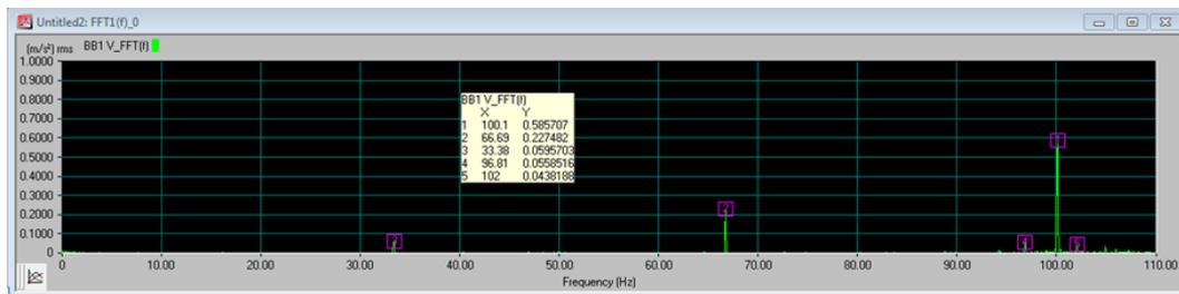
*Spectrum at Plummer block no.1 balanced 2000 rpm Vertical*
