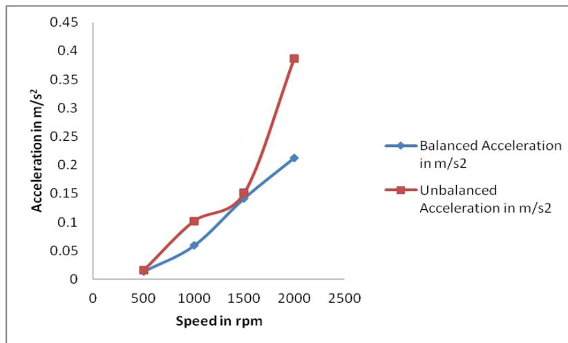
Figure8. Graph for comparison of balanced & unbalanced horizontal position
