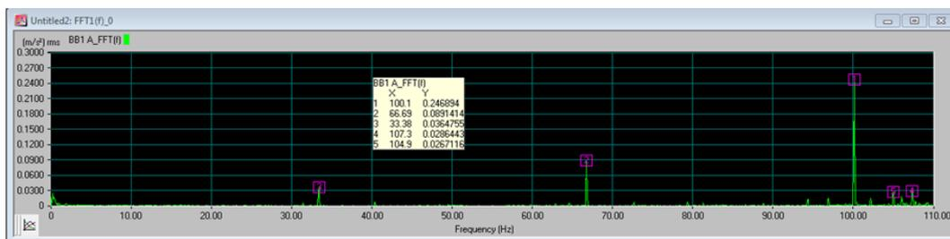
*Spectrum at Plummer block no.1 balanced 2000 rpm Axial*
