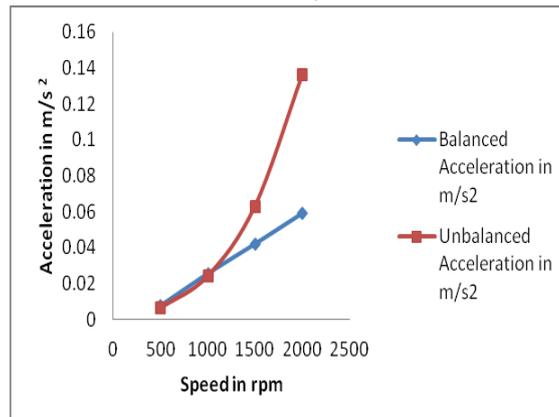
Figure 3. Graph for comparison of balanced & unbalanced vertical position
