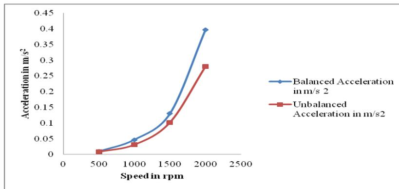
Figure7. Graph for comparison of balanced & unbalanced axial position
