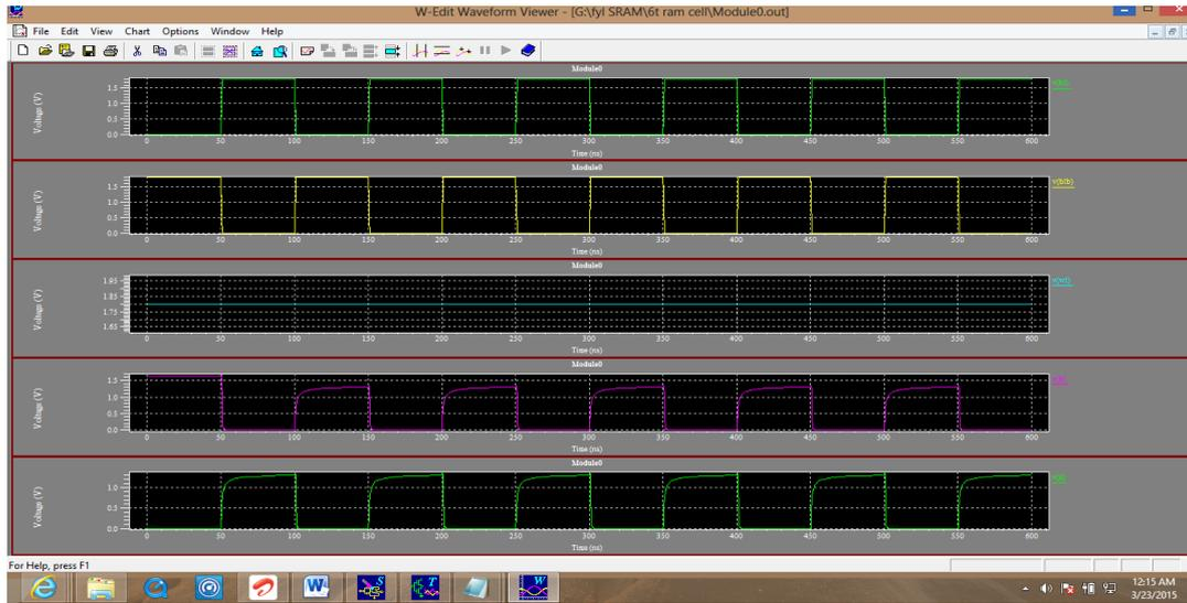
Fig6. Read/Write Waveforms of 6T SRAM Cell at 90nm
