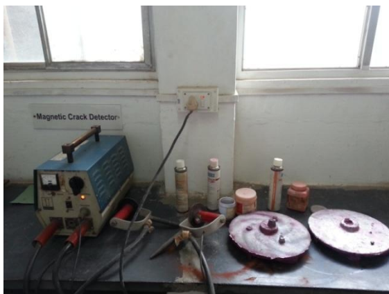
Figure1. Set Up of Magnetic Crack Detection
