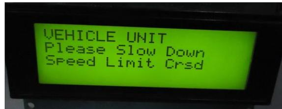
If the driver doesn't slow down the speed of the vehicle then the speed control unit in the vehicle unit will manually reduce the vehicle speed.
