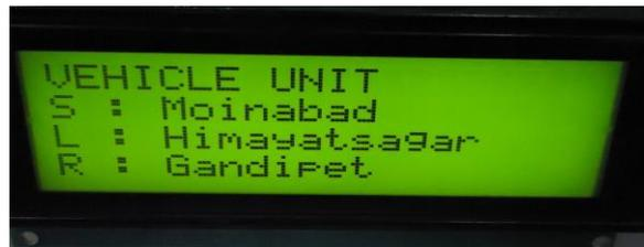
If the vehicle is going with high speed than predefined speed then the central unit will send a message to the vehicle unit to slow down the speed.
