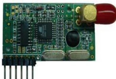
Fig. HM-TRXXX-232 RF Wireless module
