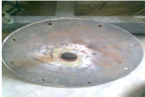
Figure6. Flange for calorimeter
