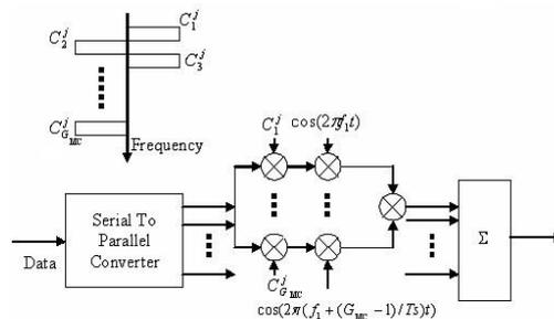
Figure1. MC-CDMA transmitter
