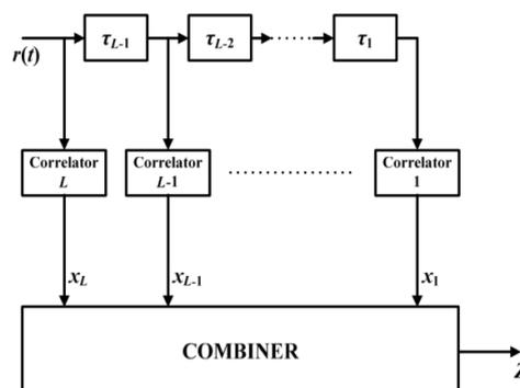
Figure2. RAKE receiver
