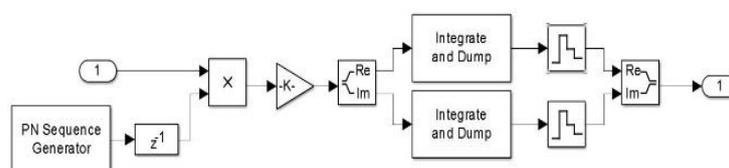
Figure5. RAKE finger Model
