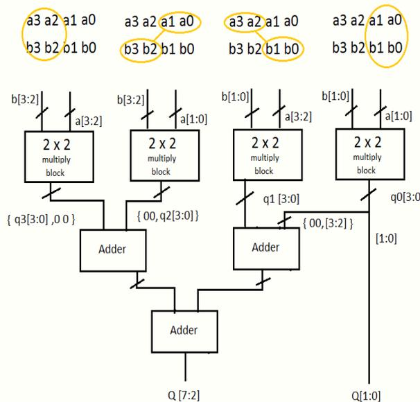
In this section a novel multiplier architecture [5] based on Urdhva Triyagbhyam Sutra of Ancient Indian Vedic Mathematics is embedded into proposed method of convolution to improve its efficiency in terms of speed and area. This method for discrete convolution using Vedic multiplication algorithm is best introduced by a basic example. For this example, let f(n) equal the finite length sequence (4 2 3) and g(n) equal the
