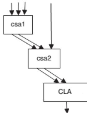
In this we are using carry save adders and cla adders in csa adder using full adders. we are having 4 bit Wallace adder first three inputs given to csa1 Sum, carry, forth input given to csa2 then sum and carry given to cla then we will get output.
