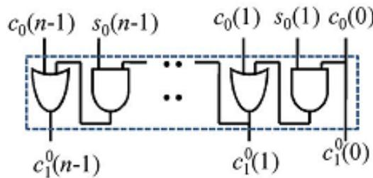
Gate-level optimized design of (CG1) for input-carry=1
