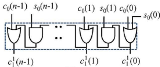
Gate-level design of the CS unit
