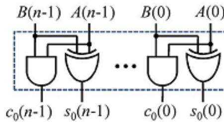
Gate-level optimized design of (CG0) for input-carry=0.
