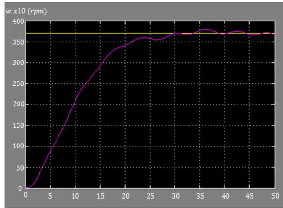
**Fig8.** Response of electric motor separately excited adapting the parameters into a PID controller based on fuzzy logic depending on mathematical models applied in Simulink®. The reference is in yellow, and the response is in magenta.
