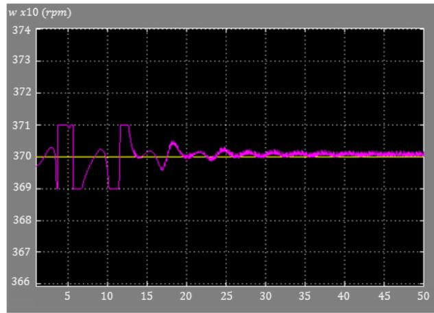
**Fig11.** Automatic PID tuning applied on Simulink® as a fuzzy logic adaptation function influenced by  $T_c$ . The reference is in yellow, and the response is in magenta.
