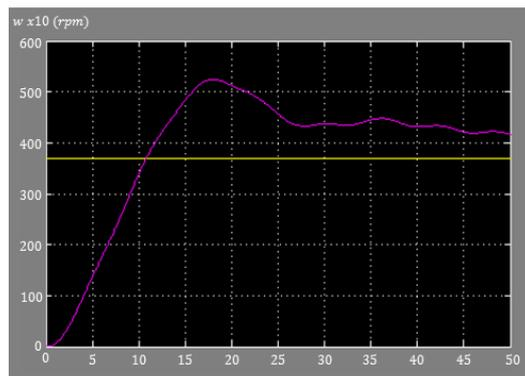
Fig5. PID controller motor with separately excited response to a step input developed into Simulink®. The reference is in red, and the response is in blue.
