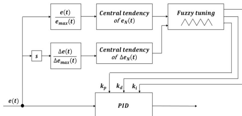
**Fig10.** Fuzzy logic PID parameters tuning block diagram.
