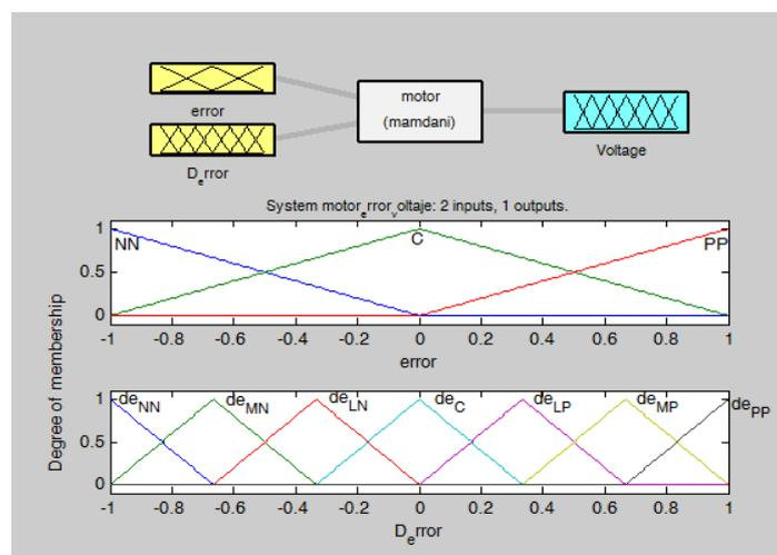
Fig7. Fuzzification based on fis module using Matlab® with Error membership functions normalized.
