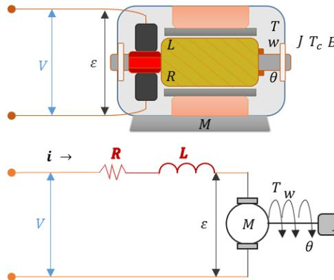
Fig2. Equivalent circuit of a permanent magnet motor.
