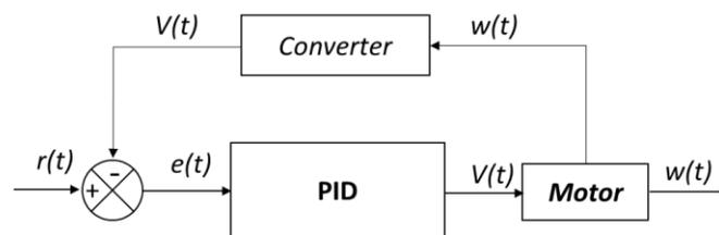
Fig4. Control block diagram for a motor separately excited.
