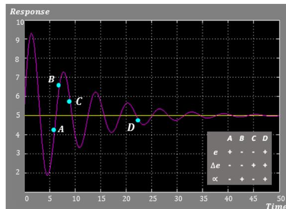
Fig1. Typical response of an underdamped second order system. The reference is in yellow, and the response is in magenta. (Information taken from Mudi (2008)).
