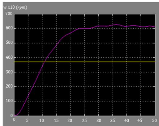
Fig3. Permanent magnet motor response to a step input without control building mathematically into Simulink®. The reference is in yellow, and the response is in magenta.
