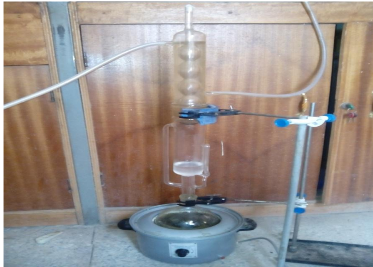
Figure2. Evaporation of Ethanol from the Extract
