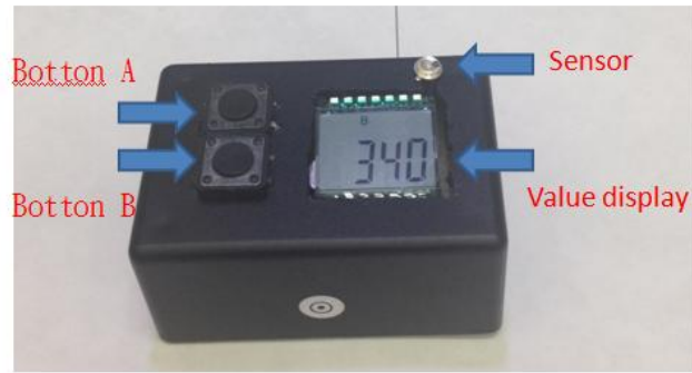
Fig4. The entity diagram of the blue light value monitor
