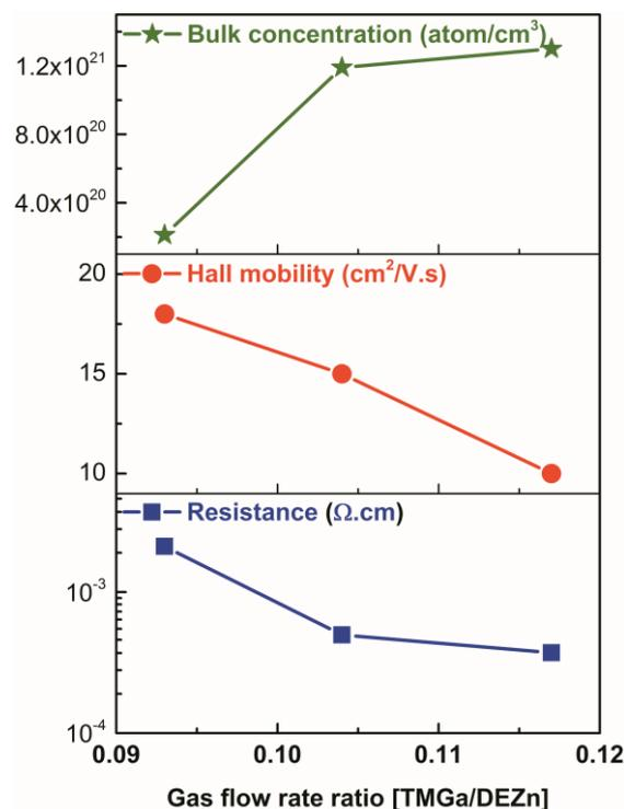
**Figure3.** Resistivity, Hall mobility, and carrier concentration as a function of gas flow rate ratio [TMGa/DEZn].
