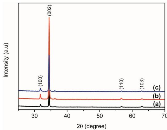
**Figure2.** XRD patterns of GZO films with various gas flow ratio [TMGa/DEZn] a) 0.09, b) 0.103, c) 0.117.
