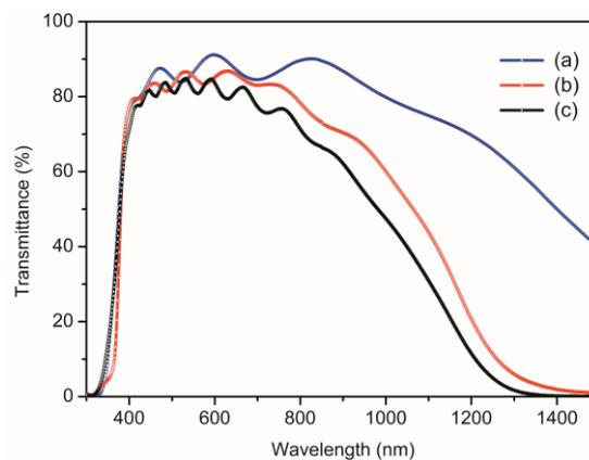
Figure4. The total transmittance of GZO films with various ratios [TMGa/DEZn] a) 0.09, b) 0.103, c) 0.117.
