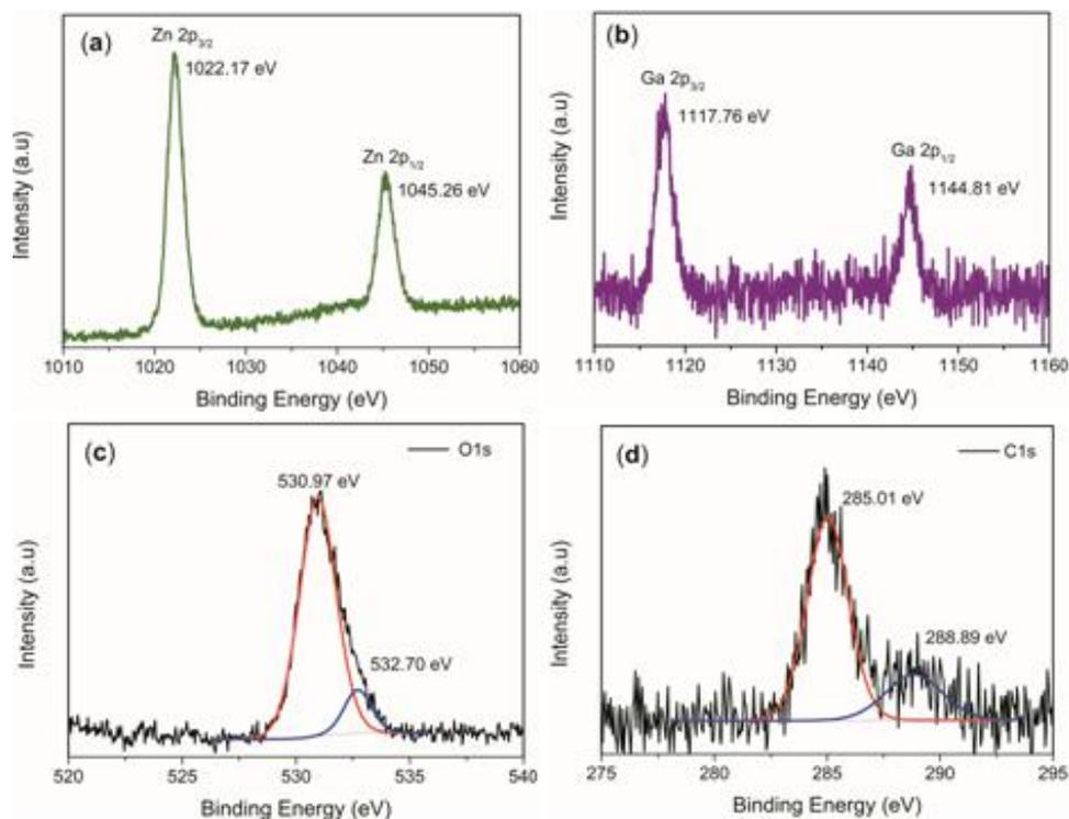
Figure5. XPS spectra of (a) Zn  $2p_{3/2}$ , (b) Ga  $2p_{3/2}$ , (c) O  $1s$  and C  $1s$  (d) for GZO films with thickness ~ 740 nm.
