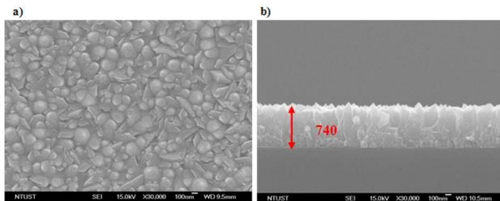
**Figure1.** SEM images of ZnO:Ga thin films a) plan view and b) cross-sectional view. The  $[TMGa/DEZn]$  ratio = 0.103.
